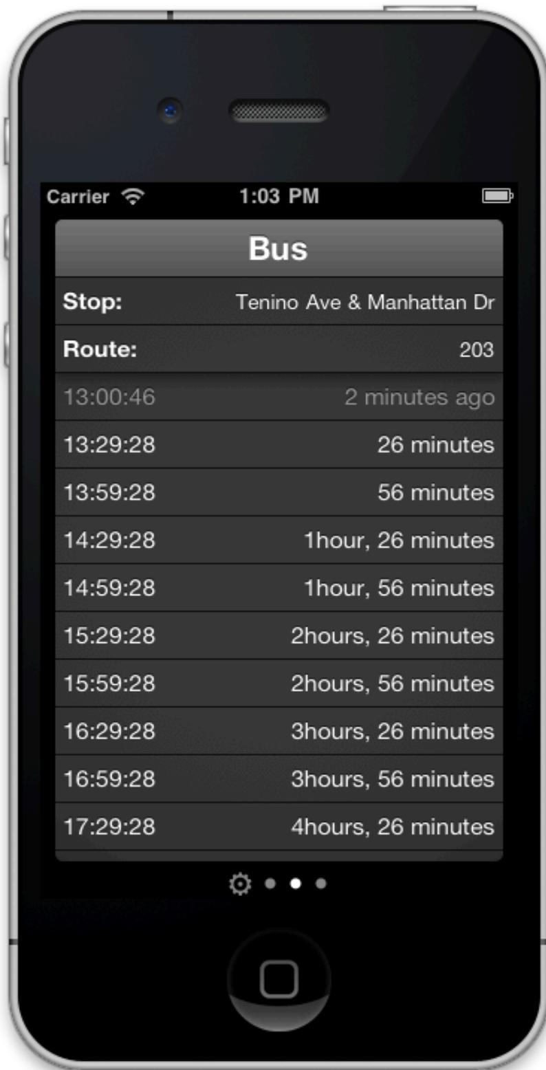
This is our Bus Widget running live. Based on the stop ID and route the user has set (seen in the settings screen), the Widget calls its DataRunner (in this case hooked up to the RTD data files) to display the upcoming times and past buses for the last thirty minutes. Data is read from data files in Google's Open Transit format, which the majority of public transportation systems nationwide use to provide data to Google Maps.
