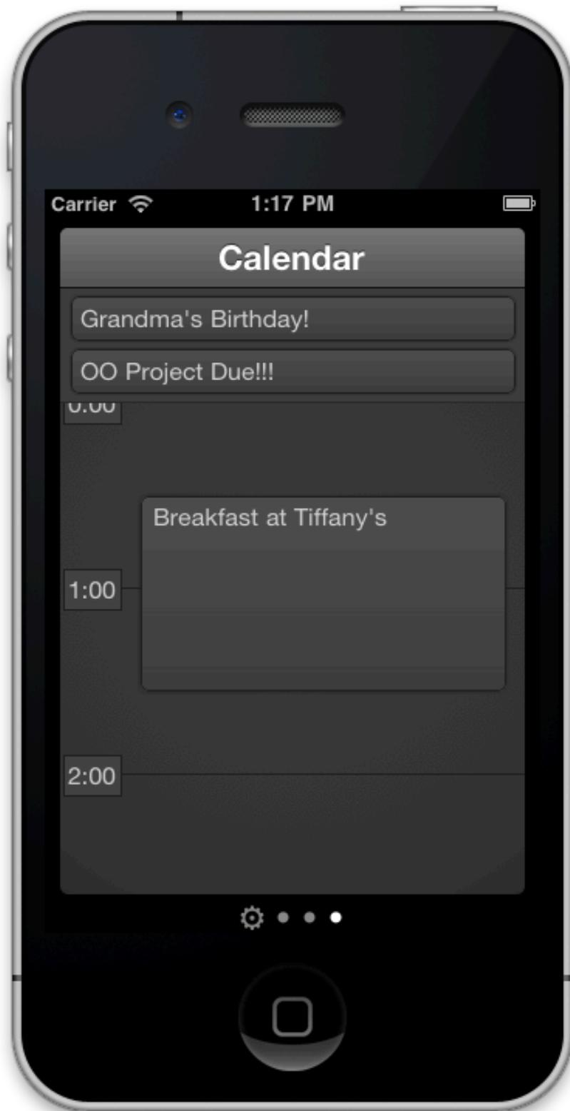
This is our Calendar widget running live. Data is pulled from the Google Calendar. Currently, the view only updates manually, but a cron job could easily be set up to run every hour, every five minutes, etc. The reason the production code does not do this is that our host, Heroku, charges for this functionality. Additionally, the reason these do not update constantly is that Google charges if we go over their free API usage.
